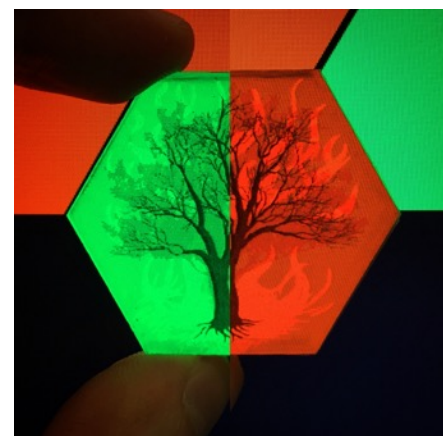
The above image shows the same printed skin for a forest fire AutomaTile over green light on the left, where the tree displays in full bloom, and over red-orange light on the right, hiding the leaves and revealing a tree set ablaze.
